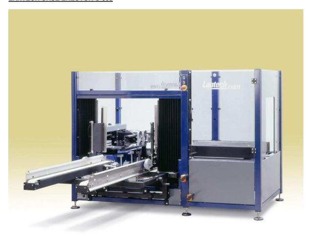
The C-300 is a case erector from the standard Lantech series. All standard equipment use proven techniques from the Lantech machine program. With this very compact case erector it is possible to handle a large number of different sizes with a high degree of reliability. Therefore the price / performance ratio is very good.
