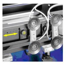
With the next movement the vacuum pick up frame hinges back to an angle of 90 degrees. This movement opens the blank to a case with open flaps. During this movement the blank is always held on two sides.
